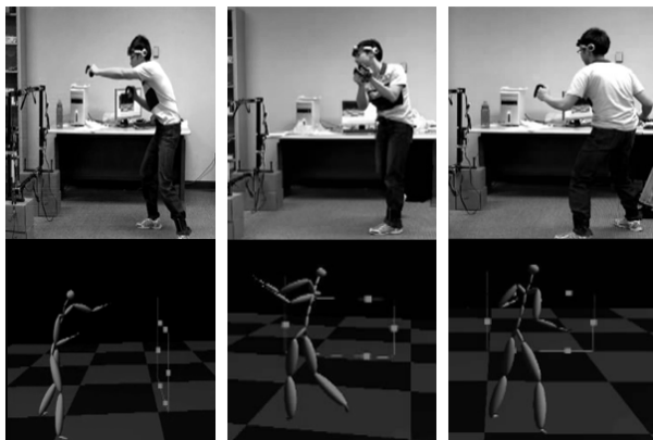
Figure 1 The actor wearing six sensors to accurately control a virtual character.
